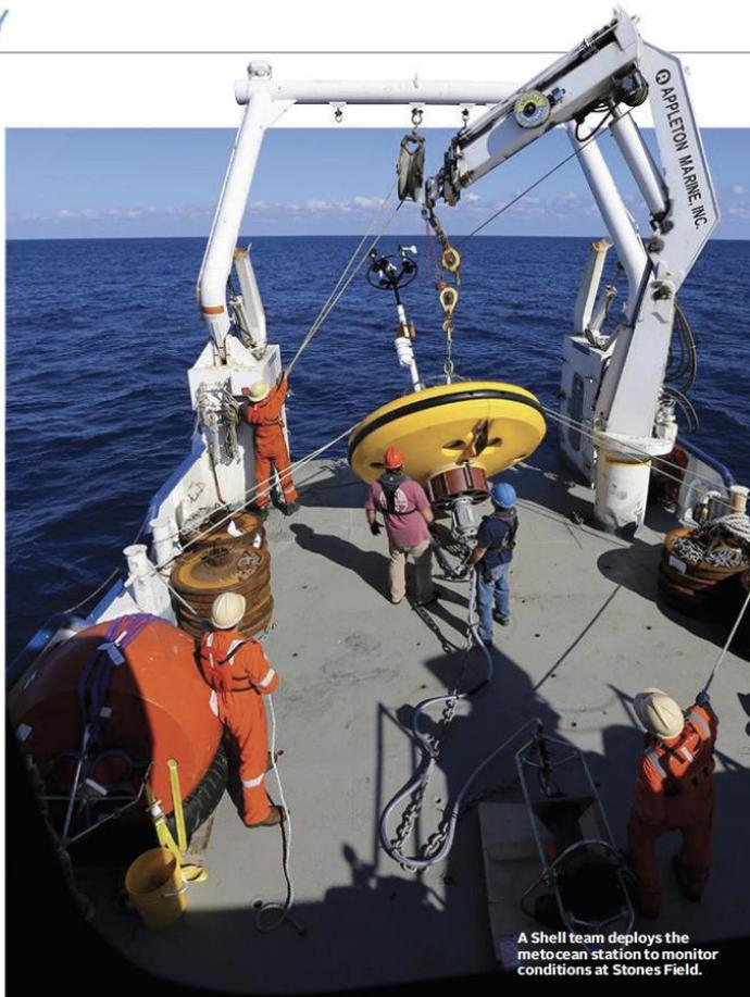
A Shell team deploys the metocean station to monitor conditions at Stones Field.
