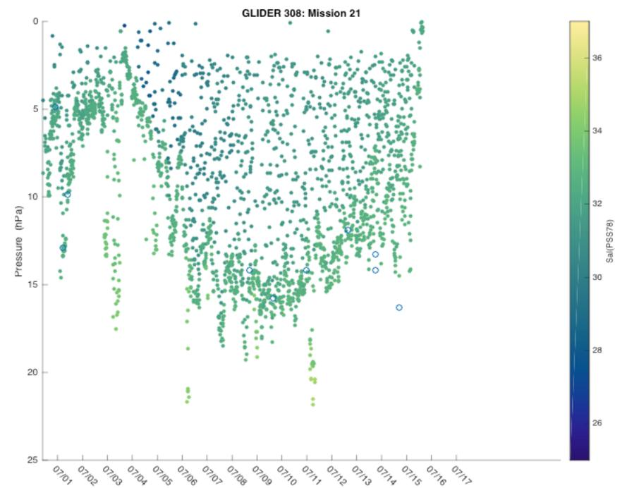
Despite being in water depths > 100 m, the glider was unable to penetrate the pycnocline at 10-15 m.
