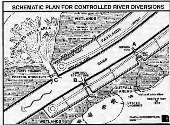
Figure 16. Schematic of three basic types of controlled river diversions: A, siphon; B, gated diversion; and C, controlled subdelta. Published with the permission of S.M. Gagliano, (51).
