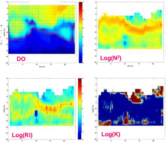
Fig. 2 24-hours continuous profile (29° N, 92° W) during August 2010. From top left to bottom right: DO concentration (black dots denote CTD measurement); B-V frequency ( $N$ ); Richardson number; vertical eddy diffusivity plotted in log scale.
