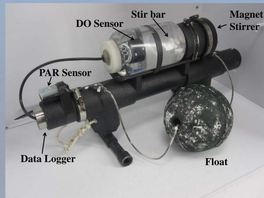
Figure 2. *In situ* incubator equipped with an Aanderaa DO optode sensor, Onset HOBO Temperature/Light Sensor, and In Situ TROLL 9500 Data Logger. Incubations were deployed for 2-6 hours in ambient light at approximately 0.25 m depth.
