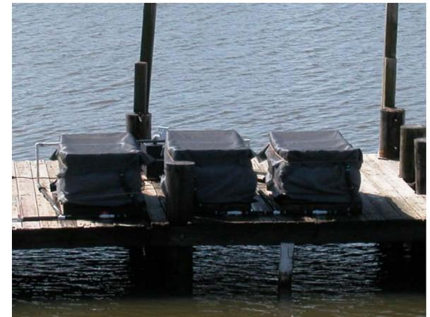
Incubators shaded to match light reaching sediment surface at each site
