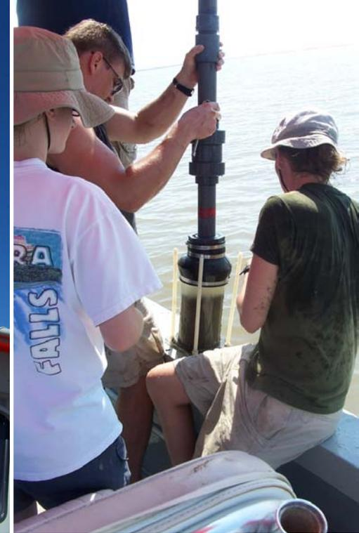
Triplicate sediment cores and “short” bottom-water cores incubated in dark (light doesn't reach sediments) at ambient temperatures
